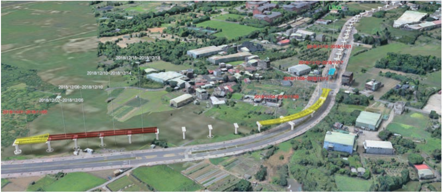
3D GIS-assisted Construction Progress of the New Taipei City MRT SanYing Line Project Planning and Turnkey Project, Showing the Completion, Construction in Progress, and Prospective Three Construction Phases
