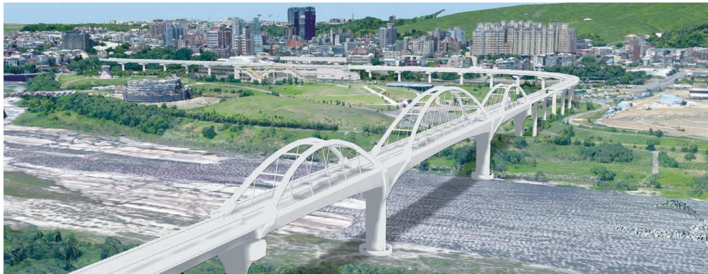
Result of integrated SanXia River Bridge BIM Model with 3D Reconstructed Model of the New Taipei City MRT SanYing Line Project.
