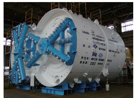
First Double O-Tube (DOT) tunnelling in Taiwan
